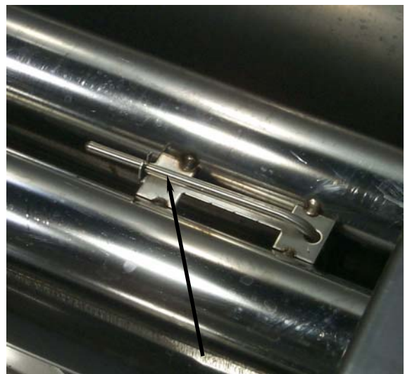
Electronic thermostat probe in frypot (arrow).
